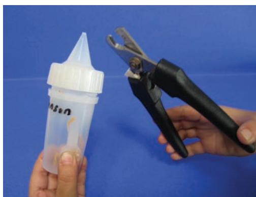
3. Cut nozzle off with nail trimmer.
